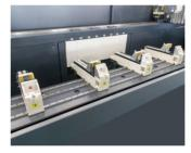
The GARNET XS4, which positions its clamps fully automatically using the X-axis, completely takes on the user's workload.
