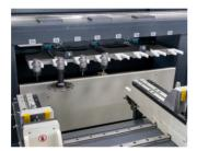
Thanks to its built-in automatic magazine with capacity for 8 tools, GARNET XS4 saves time when switching to different operations.
